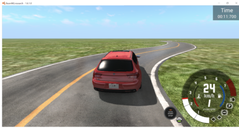
Figure 4: A test case rendered by the BeamNG simulation engine is composed by the road, the driving task, the environment and the car
